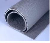
Our **CT-190** is heavy 32 oz fiberglass cloth coated with a grey mastic covering. Its use is the similar to the CT-4000 cloth but it offers a little more protection because of the thickness of the cloth. It is recommended as a heat shield
