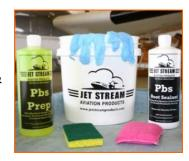
STEP 1, CLEANING BOOTS: Put on latex gloves. Apply the **Pbs Prep** directly to the scrubbing sponge as shown in photo. Using the soft side of the sponge, apply the **Pbs Prep** to the de-ice boot. By keeping the de-ice boots wet with **Pbs Prep** for 2-3 minutes all old boot treatments will begin dissolving. At this point use the scrubbing side of sponge to help remove old boot treatments. De-Ice boot should now be ready for rinsing.
