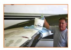
STEP 3, APPLYING PBS BOOT SEALANT: Apply Pbs Boot Sealant directly on a clean micro fibre applicator. Using the treated micro fibre applicator, apply the Pbs Boot Sealant to de-ice boot in one direction. Apply 3-5 coats allowing each coat to dry before applying the next quote. When the de-ice boot is completed, it will have a wet glossy appearance, but will be dry to the touch.
